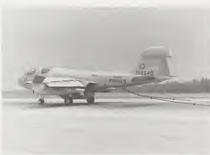
A Marine EA6B, weighing 20 tons and landing at a speed over 120 miles per hour, slams to a stop in a few hundred feet by catching an arresting cable. Marines have developed portable arresting gear systems that can be installed in a few hours.
