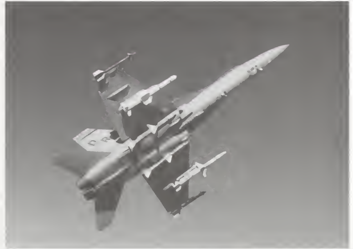
A Marine F/A-18 armed with a variety of missiles including a HARPOON. Only Navy/Marine Corps aircraft can fire this sophisticated anti-ship missile. (Photo courtesy of McDonnell Douglas Corporation.)
