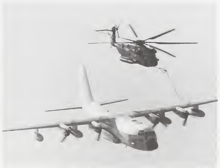
A CH-53 Sea Stallion refuels from a Marine KC-130 Hercules. CH-53E's have played a vital role in a wide range of operations, including the rescue of non-combatants from the American embassy in Somalia in 1991.
