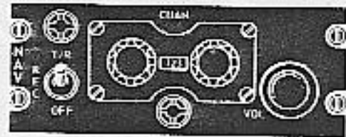
TACAN CONTROL PANEL (ASC 36 installed)
