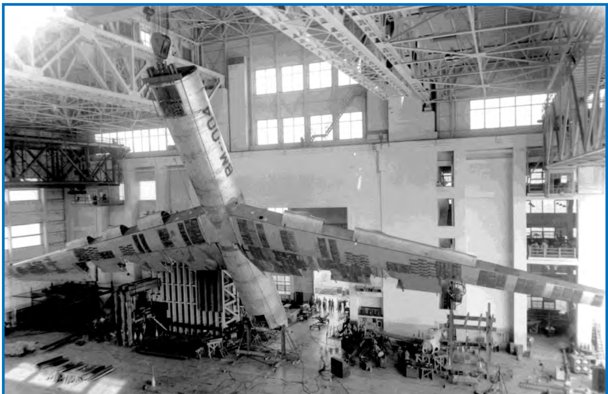
All: The first B-36A (44-92004), became the static test article for the B-36 fleet. This aircraft made just two flights in August 1947, one local flight around Fort Worth to prove its airworthiness and a flight to Wright-Patterson AFB, OH where the aircraft underwent structural testing in a variety of positions until tested to destruction (below). Prior to its first flight, the aircraft is displayed at an Army Air Forces Day Open House at Carswell AFB on August 3, 1947 (above).
