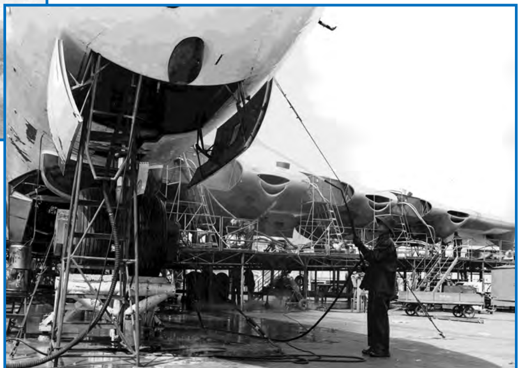
Right: Decontaminating a Peacemaker after a nuclear test is a manpower intensive task. Workers scrubbed the aircraft with a mixture of Gunk and kerosene followed by plenty of water. Note the lack of proper protective gear.
