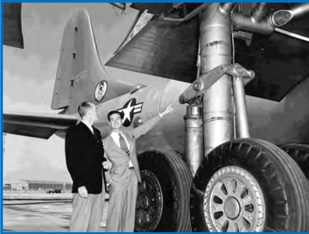
Top: Convair executives examine the main landing gear of the B-36 Peacemaker .
