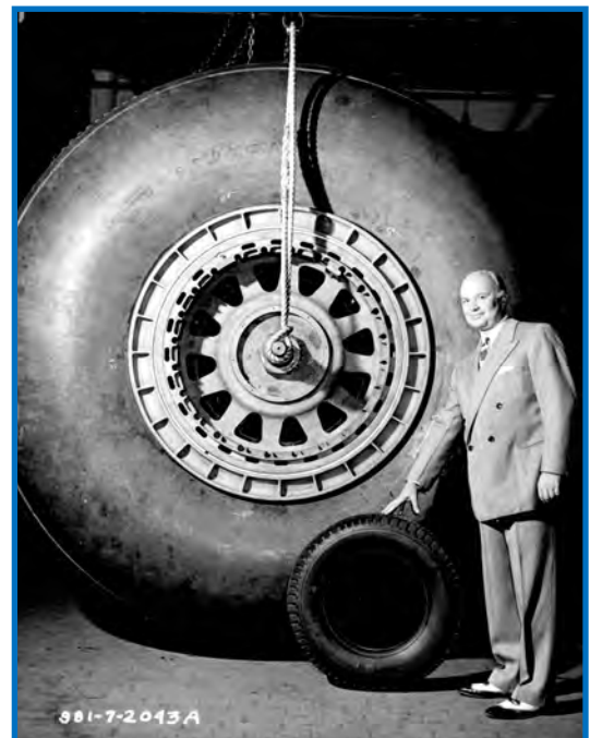
Bottom: Mr. E. J. Thomas, President of Goodyear Tire & Rubber Company with 6.00 x 16 auto tire and the 110-inch XB-36 tire.
