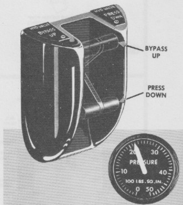
Figure 1-28. Hydraulic Pressure Bypass Handle and Hydraulic Pressure Gage
