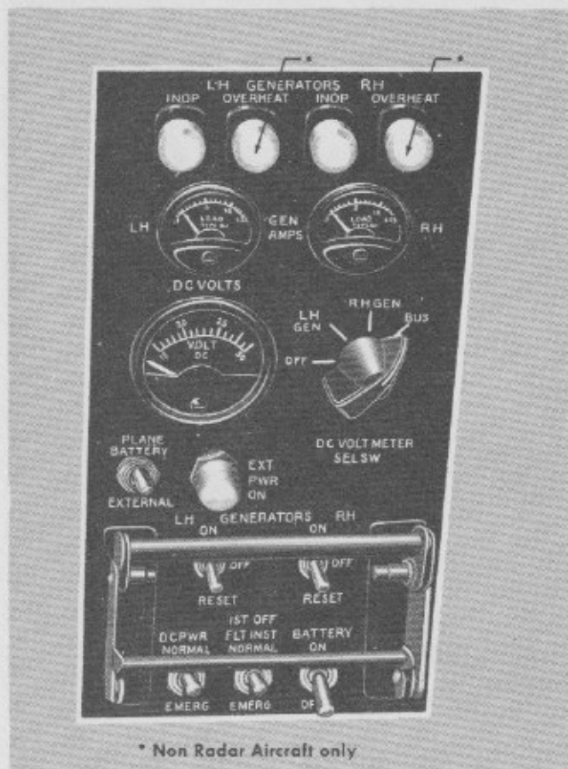
Figure 1-22. DC Control Panel
